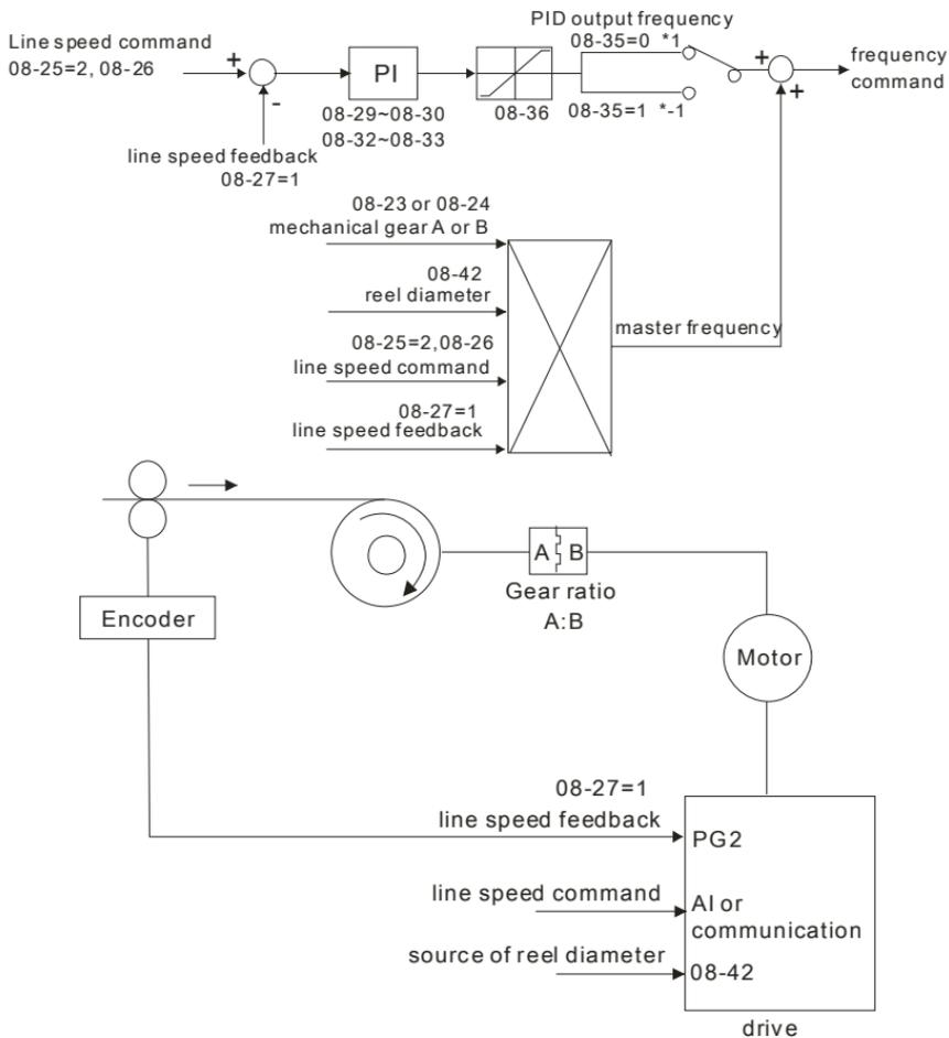
4: Tension open-loop, torque mode
