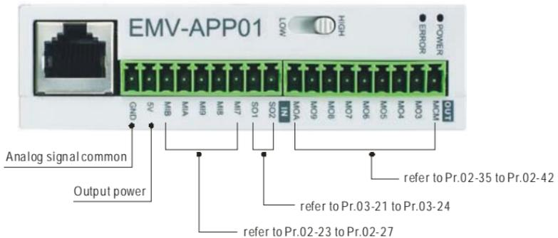
When wiring, please refer to the multi-function input/output function in parameters group 02 and group 03 of chapter 4 parameters to set by your applications.
