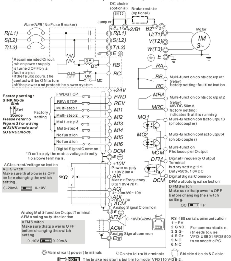
Figure 2 for models of VFD-VE Series (15HP/11kW and above)
