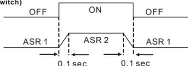
**10-09** ✓ Low Pass Filter Time of ASR Output
