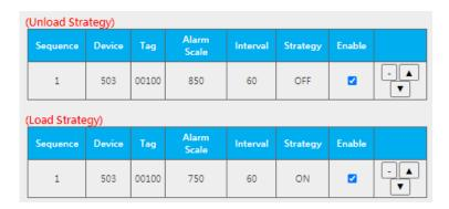
Unload and load type indicates that the value is greater or lower than alarm scale. Strategy is set to turn on or off the specific device, or input values.
