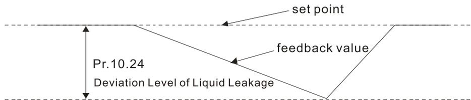
**10.25** Liquid Leakage Change Detection
