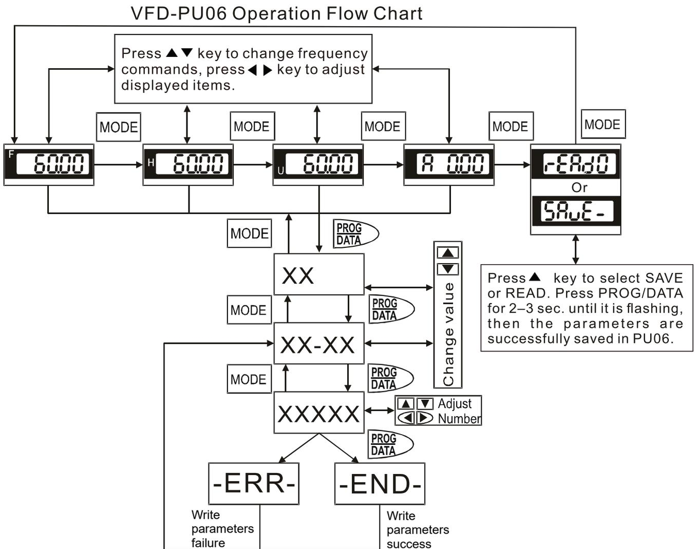
B-3-2 Digital Keypad VFD-PU08 / VFD-PU08V
