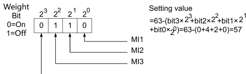
**04.27** Internal/ External Multi-Function Input Terminal Selection
