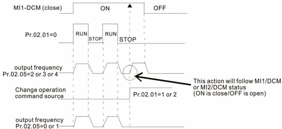
When you set Pr.02.05 = 1 or 3, it does not guarantee that the drive will never run. Be careful when using this function because the switch may bounce due to mechanical vibration or defective switch parts.
