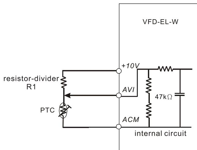
Take the standard PTC thermistor as an example: if the protection level is 1330 Ω, the actual voltage between +10V-ACM is 10.5 V and divider resistance R1 is 4.4k Ω.
