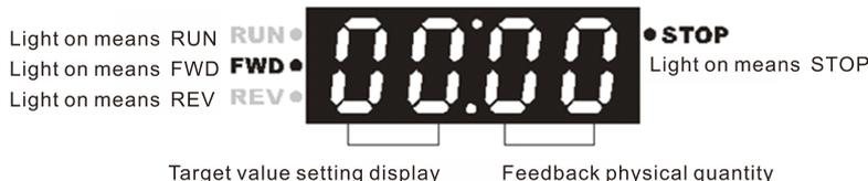
In the flow control occasions such as constant pressure water pumps using PID control, set Pr.00.03 = 3 and Pr.00.04 = 8. When the drive reboots after powered off, the start-up screen displays 00:00 (as shown in the figure above). The displayed value on the left of “:” is the physical quantity of PID target value; on the right of “:” shows the sensor output value (0–10V/4–20 mA) corresponding to the actual physical quantity.
