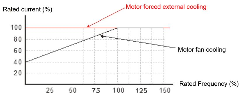
**06.07** Electronic Thermal Relay Action Time
