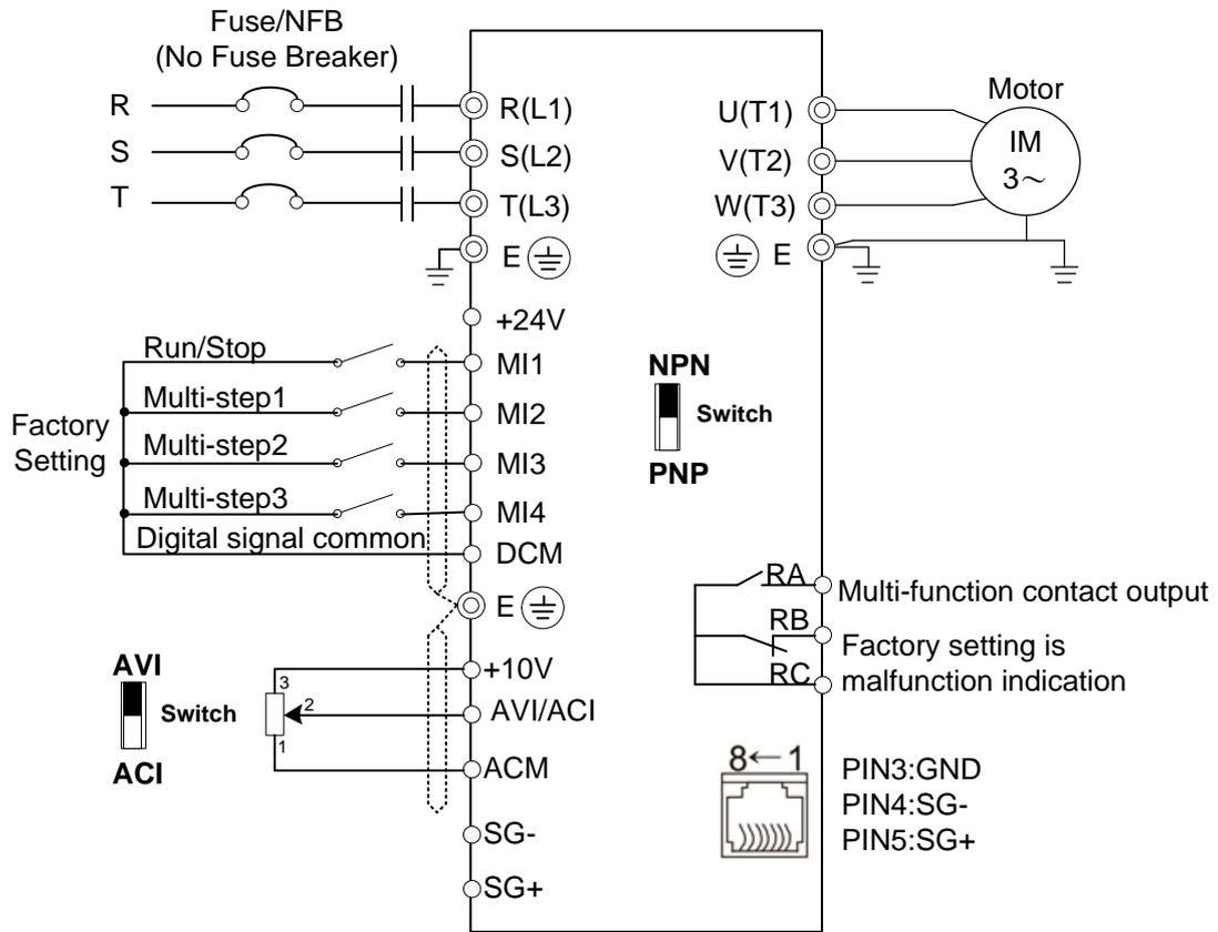
⊙ Main circuit (power) terminals   ○ Control circuit terminals   Ⓢ Shielded leads & cable
