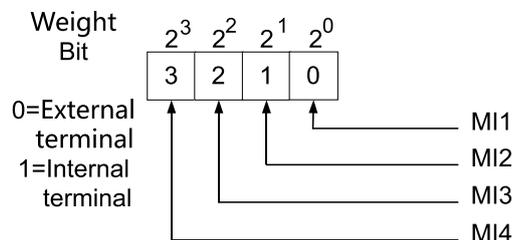
When setting this parameter, convert bit3–bit0 that represent the status of MI4–MI1 from binary to decimal, and then set this parameter. Set MI3 and MI4 as internal terminals; set MI1 and MI2 as external terminals. Pr.04.27 should be set to 12.
