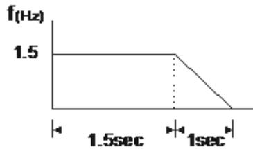
Therefore, the motor's operation distance after executing the stop command = number of revolutions  $\times$  circumference =  $1.5 \times 2 \pi r$ . It also means that the swivel table stops after running 1.5 revolutions.
