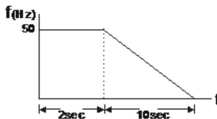
Therefore, the motor's operation distance after executing the stop command = number of revolutions  $\times$  circumference =  $175 \times 2 \pi r$ . It also means that the swivel table goes back to the top after 175 revolutions.
