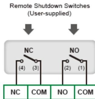
(Figure 4-29: REPO Dry Contacts\_ Pins<sup>1</sup> Location and Wiring Diagram)
