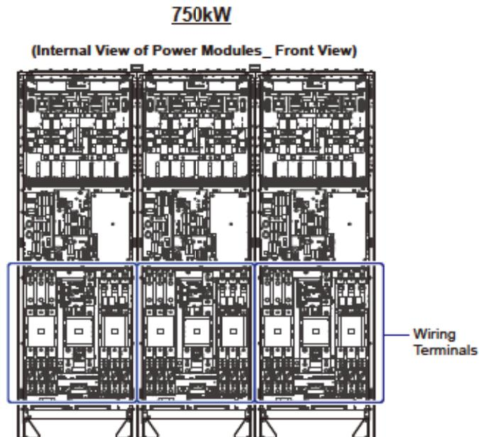
(Figure 2-13: Location of the Power Modules' Wiring Terminals)
