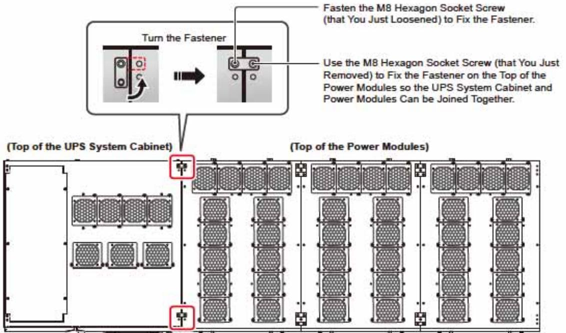
(Figure 5-6: Turn the Two Fasteners and Use the Two Fasteners to Join the Top of the UPS System Cabinet and the Top of the Power Modules Together)
