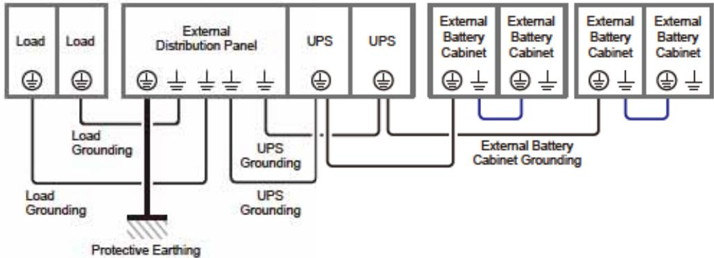
(Figure 5-40: Grounding Diagram\_ Parallel Units)
