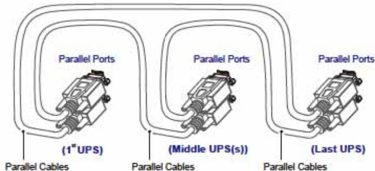
(Figure 5-35: Parallel Ports Connection among the Parallel UPSs)
