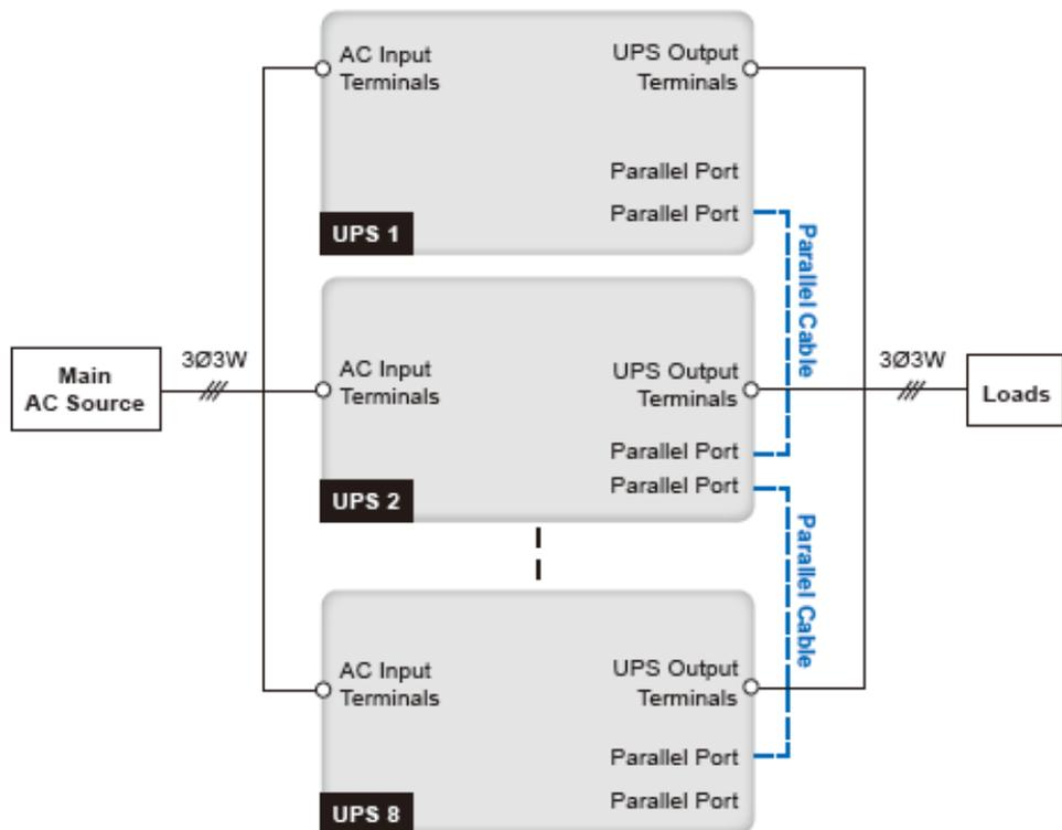
(Figure 5-34: Parallel Units Single Input Wiring Diagram)
