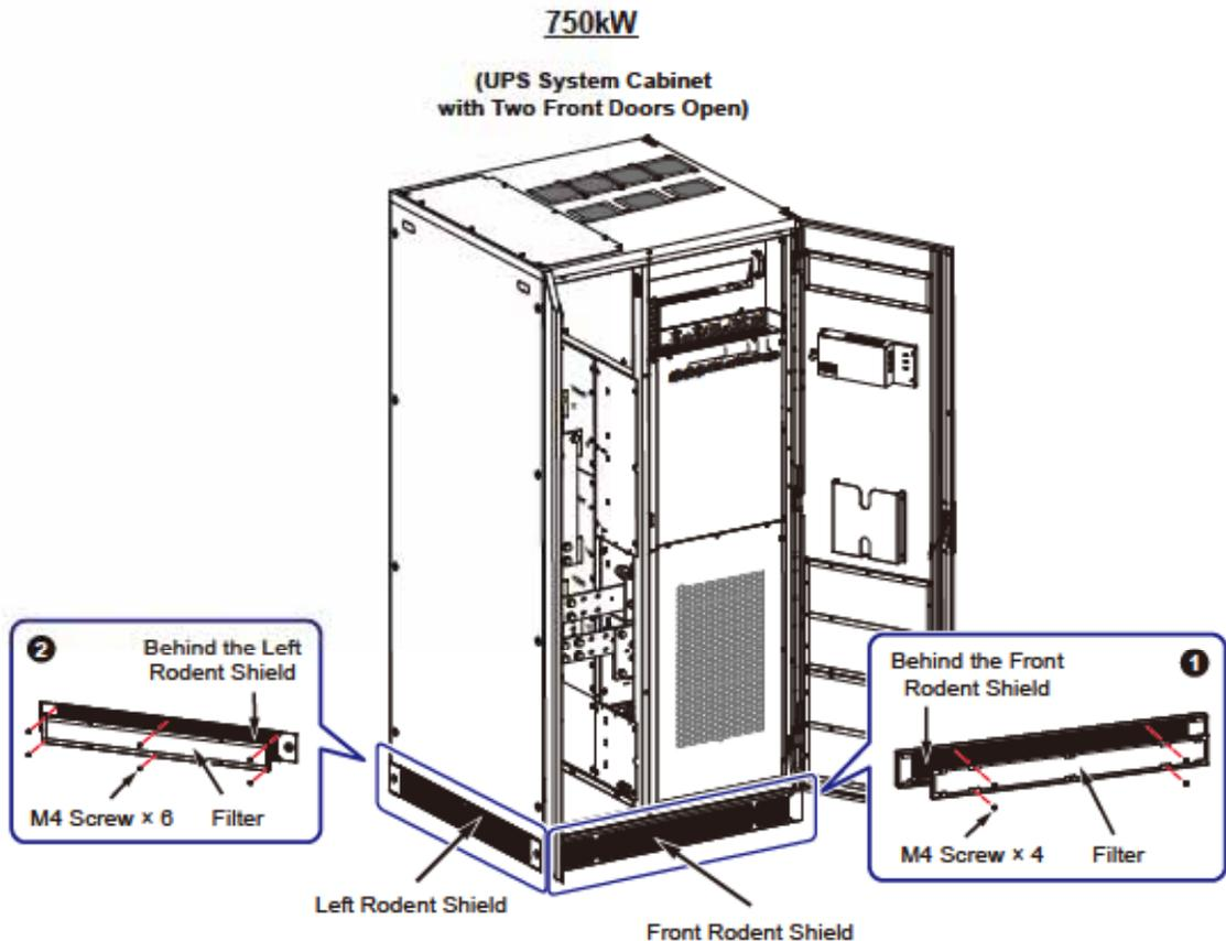
(Figure 9-7: Dust Filters Located behind the UPS System Cabinet's Front & Left Rodent Shields)
