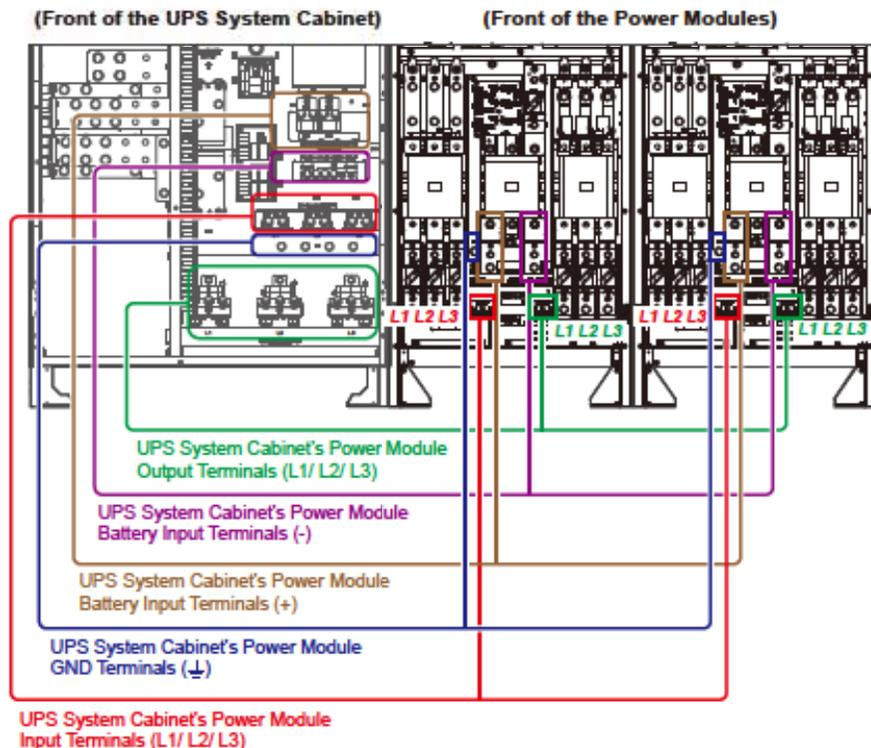
(Figure 5-26: Internal Wiring between the UPS System Cabinet and the Power Modules\_ 500kW UPS)
