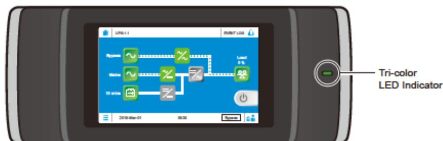
(Figure 2-17: Tri-color LED indicator Location)
