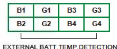
(Figure 4-23: External Battery Temperature Detection Dry Contacts)
