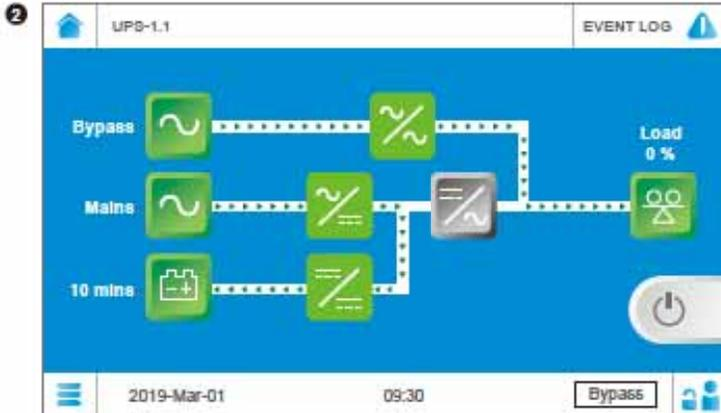
The screen above indicates that the UPS is in **Bypass** mode and the inverter is off. Please refer to **6.2.3 Bypass Mode Start-up Procedures**.
