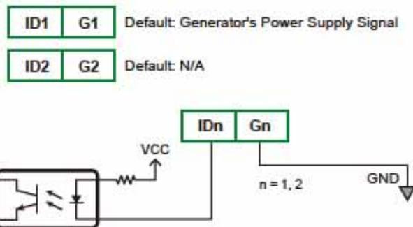
(Figure 4-26: Input Dry Contacts\_ Pins<sup>1</sup> Location and Wiring Diagram)
