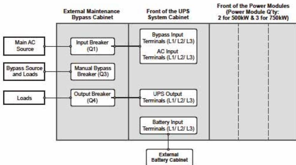
(Figure 5-31: Single Unit Single Input Wiring Diagram)
