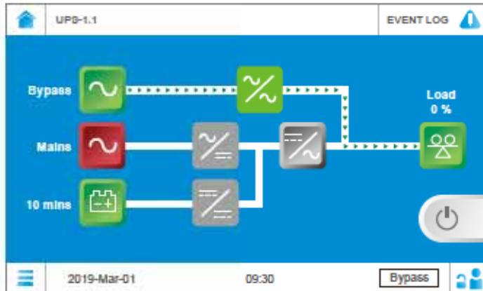
Next, turn OFF the external maintenance bypass cabinet's output breaker (Q4) and each external battery cabinet's breaker (Q5). At this moment, the tri-color LED indicator still illuminates yellow.
