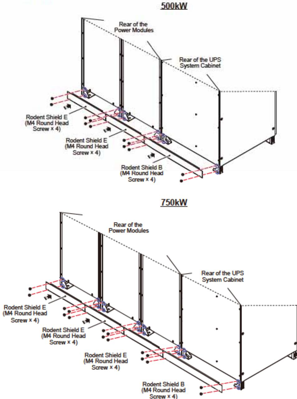
(Figure 5-15: Install the Rodent Shields at the Rear Bottom of the UPS System Cabinet and the Power Modules)
