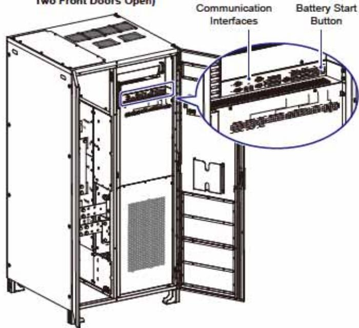
(Figure 7-2: The Position of Battery Start Button)
