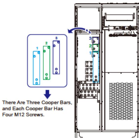
(Figure 5-20: Location of the Three Copper Bars & M12 Screws)
