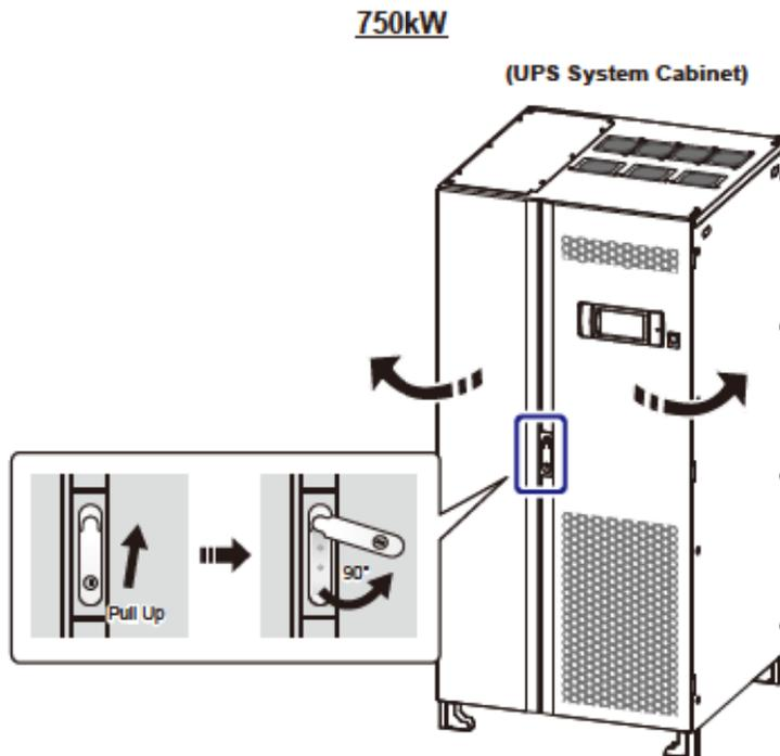
(Figure 2-7: How to Open the UPS System Cabinet's Two Front Doors)
