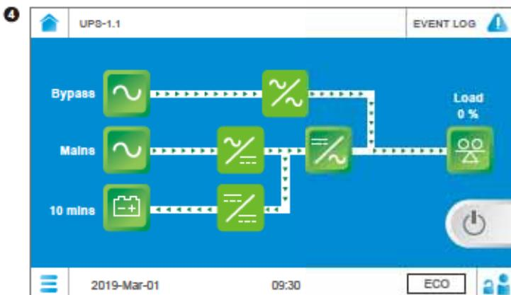
The screen above indicates that the UPS is in ECO mode. The inverter is in the ready-to-power-on status, and the power supply of the loads comes from the bypass. For ECO mode settings, please refer to **7.9.2 Mode Setting** and **6.2.5 ECO Mode Start-up Procedures**.
