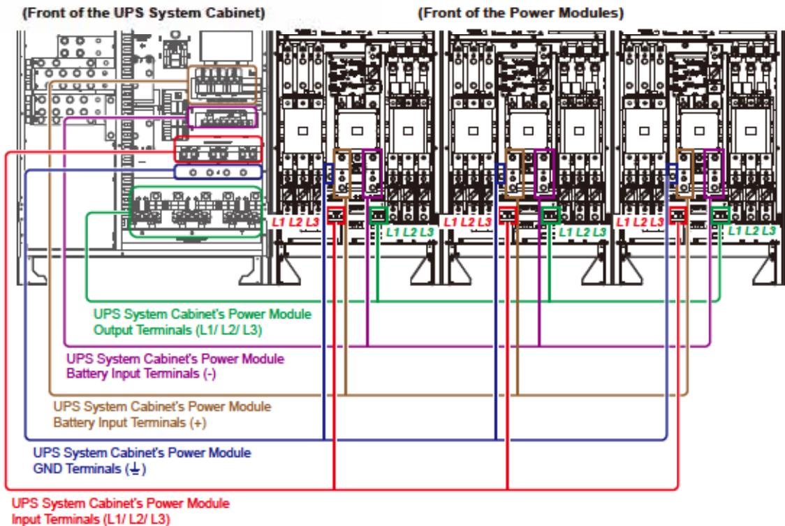
(Figure 5-28: Internal Wiring between the UPS System Cabinet and the Power Modules\_ 750kW UPS)
