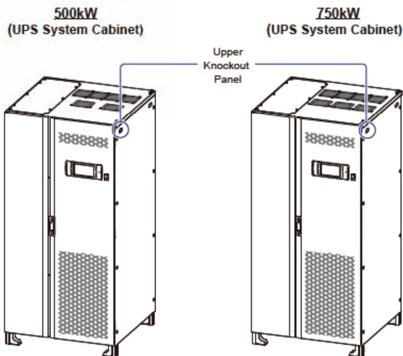
(Figure 5-2: Knockout Panel Location of the UPS System Cabinet)
