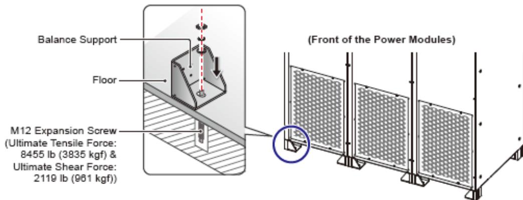
(Figure 5-9: Balance Support Installation Method for the Power Modules)
