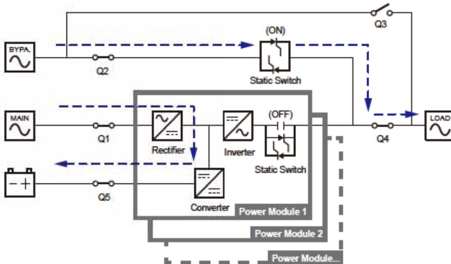
(Figure 3-3: Bypass Mode Diagram)
