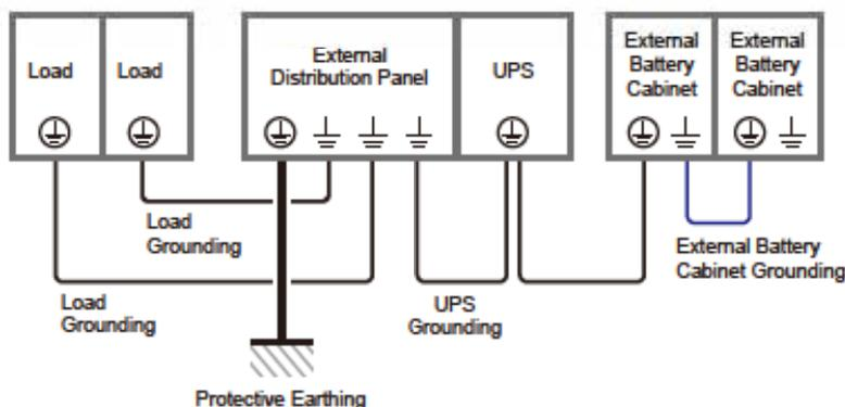
(Figure 5-32: Grounding Diagram\_ Single Unit)
