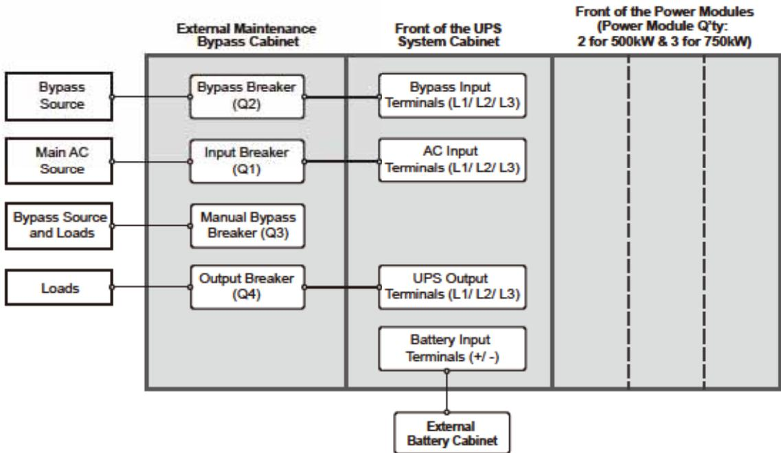
(Figure 5-33: Single Unit Dual Input Wiring Diagram)
