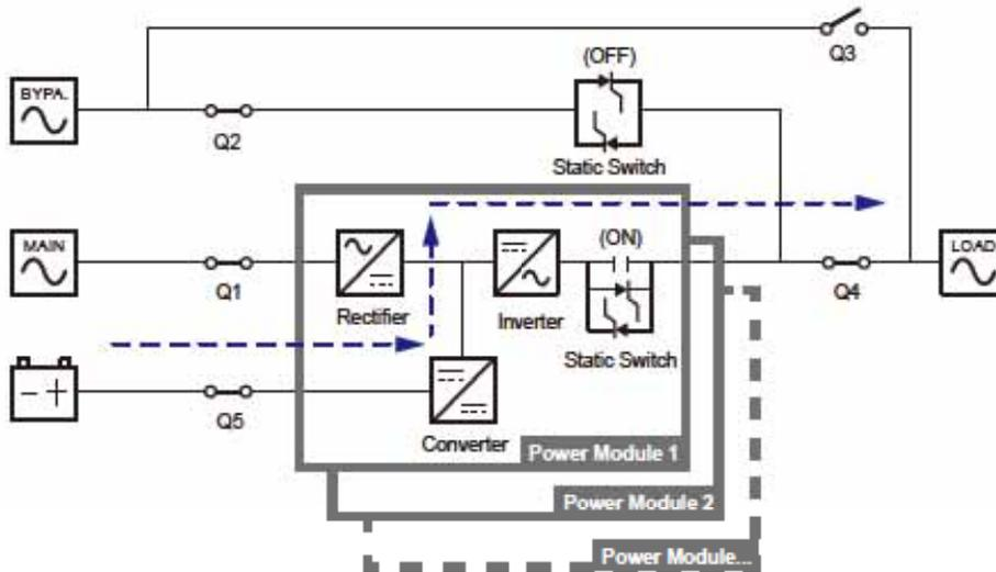
(Figure 3-2: Battery Mode Diagram)
