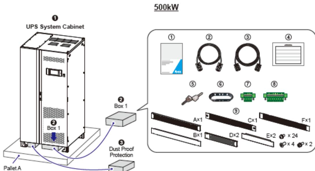
(Figure 2-1: Pallet A, UPS System Cabinet & Box 1)
