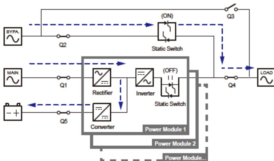
(Figure 3-5: ECO Mode Diagram)
