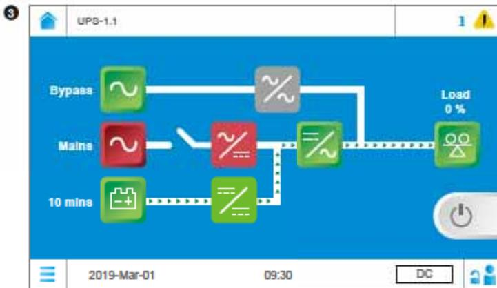
The screen above indicates that the UPS is in **DC** mode, and power supply of the loads comes from the batteries. Please refer to **6.2.2 Battery Mode Start-up Procedures**.
