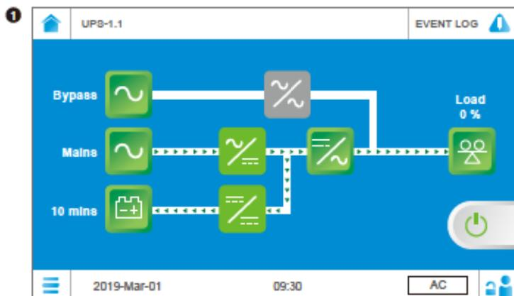
The screen above indicates that the UPS is in **AC** mode, and power supply of the loads comes from the inverter. Please refer to *7.9.2 Mode Setting* and *6.2.1 On-Line Mode Start-up Procedures*.
