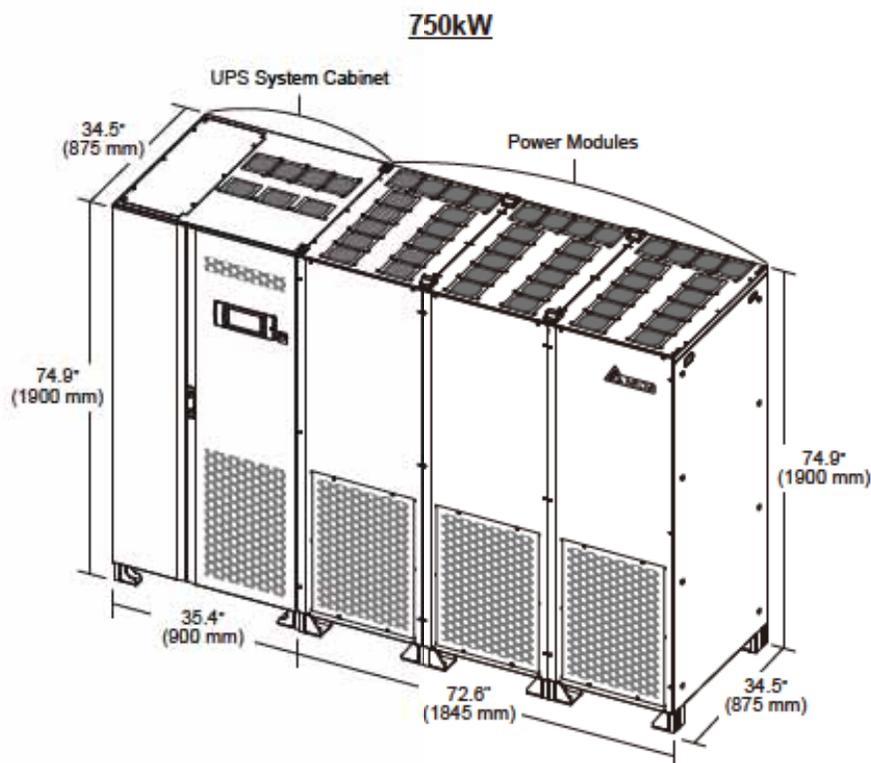
(Figure 2-5: UPS Exterior & Dimensions)
