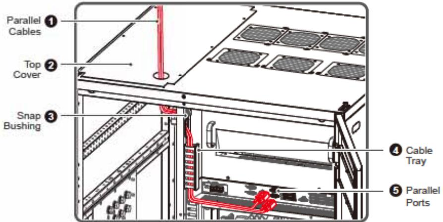
(Figure 5-37: Top Entry & Location of Parallel Cables, Top Cover, Snap Bushing, Cable Tray and Parallel Ports)
