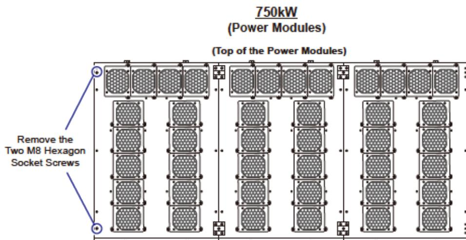
(Figure 5-5: Remove the Two M8 Hexagon Socket Screws Located on the Top of the Power Modules)
