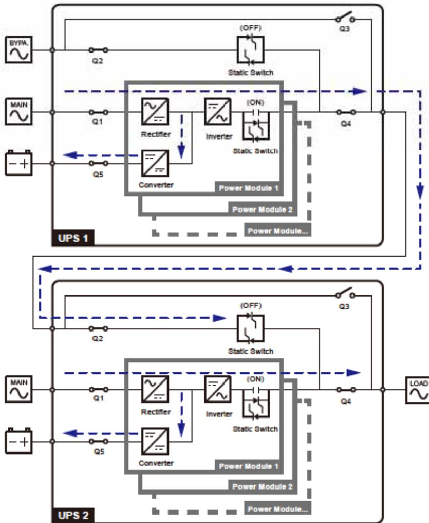
(Figure 3-6: Hot Standby Redundancy Diagram (only for Dual Input & at Least Two UPSs))
