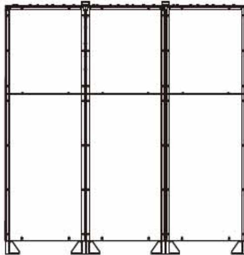
(Figure 2-15: Rear View of the Power Modules)
