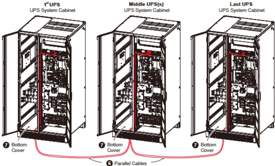
(Figure 5-38: Top Entry\_ Parallel Cables Routing)
