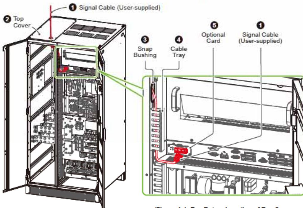
(Figure 4-3: Top Entry\_ Optional Card's Signal Cable Routing)
