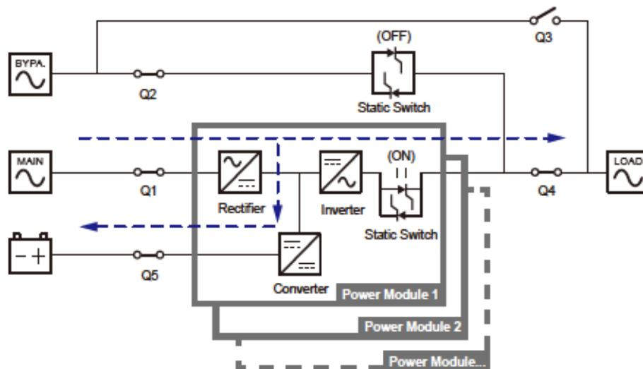
(Figure 3-1: On-Line Mode Diagram)
