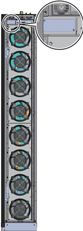
(Figure 3-8: RowCool—chilled water type (HCH1840/HCH1850): SNMP card slot location)
