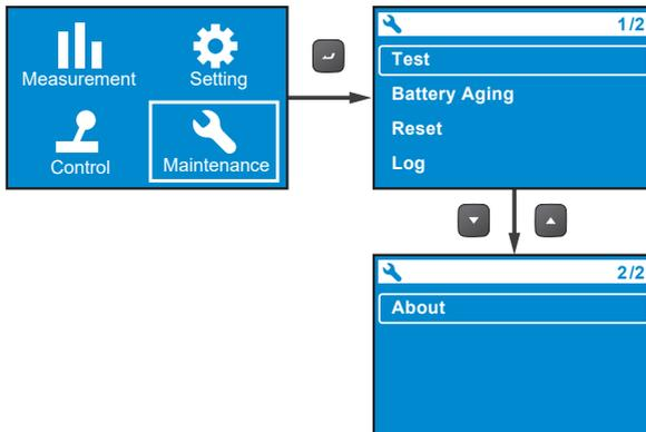
The **Maintenance Menu** provides commands for enabling UPS maintenance functions. It also provides event logs and UPS identification. Please refer to the table below for the setup items and selectable values.
