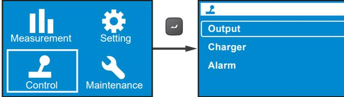
The **Control Menu** provides commands for enabling specific UPS functions. Please refer to the table below for the setup items and selectable values.
