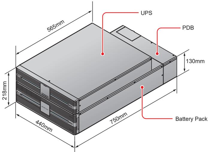
(Figure 2-2: Standard Runtime Model - 8/ 10KVA Exterior & Dimensions)
