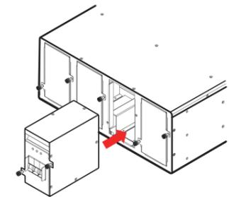
**NOTE:** If you want to install two 30A or 32A breaker modules (optional), it is necessary to install the breaker modules at an interval of one slot with the slot cover installed. Please refer to the figure below.
