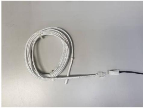
(Figure 3-16: Leakage Detection Sensor & Connector)
